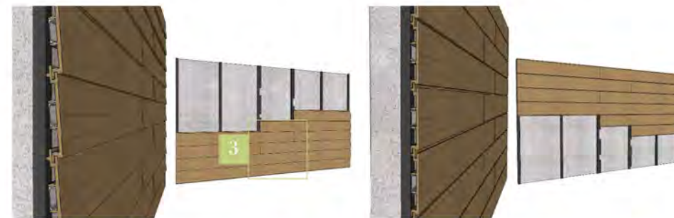
EWP-180U Multi-function exterior wall panel schematic drawings EWP-180U多功能外牆板示意圖
